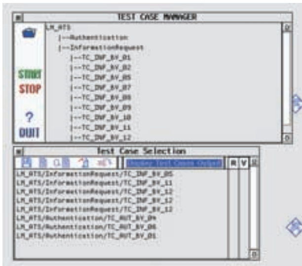
FIG 3 Any sequences and repetitions of test cases can be combined in the test case manager
