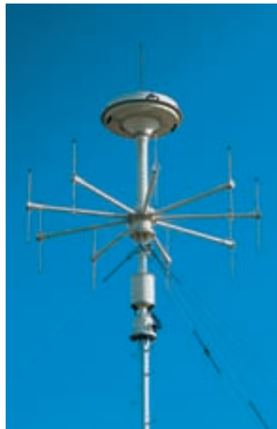
FIG 3 Together, correlative interferometer antennas ADD 051 (= ADD 050 with ADD 150) and ADD 070 (cylinder below) cover the frequency range 20 MHz to 3000 MHz
