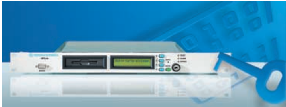
FIG 1 SITLink for confidential communication on synchronous leased lines up to 2 Mbit/s
