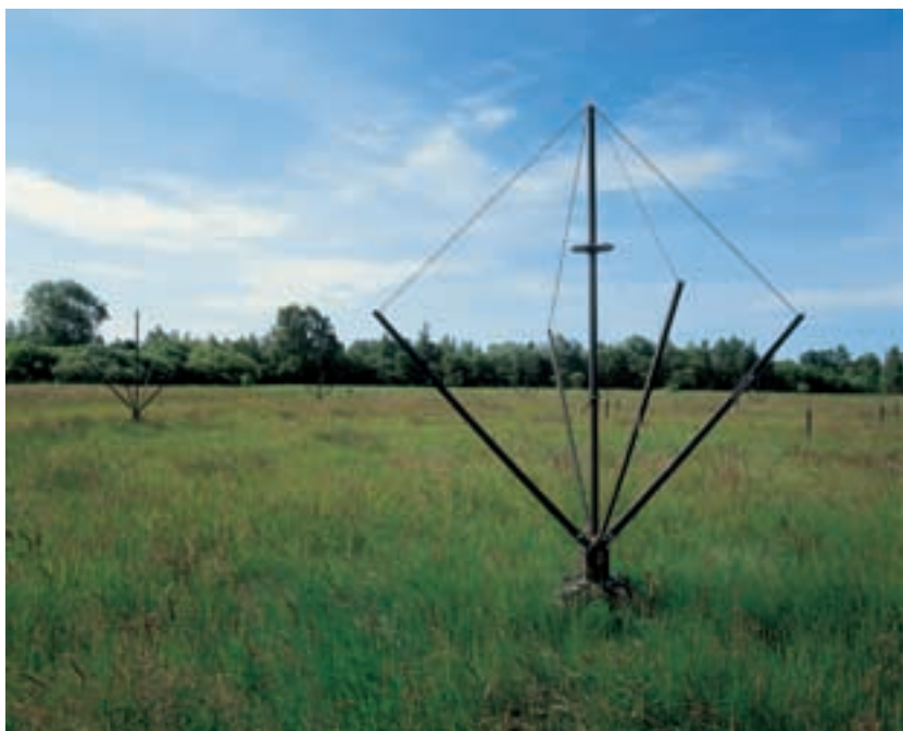
FIG 1 Interferometer DF Antenna ADD011, combined with Adcock Antenna ADD012 (monopoles in background, right)
