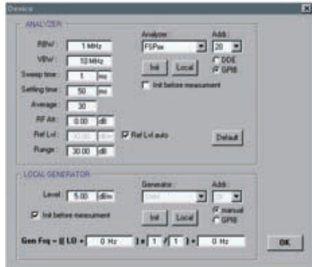
FIG 2 Setup of FSP with Noise Measurement Software FS-K3 (set sweep time set to 1 ms and average to 30 for example, deactivate "Init before measurement")
